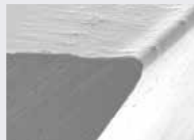
An uncoated High Speed Steel cutting edge is already rounded after cutting only 1000 m of Spruce.
