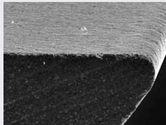
A conventional High Speed Steel cutting edge is already round after cutting only 1000 m of Spruce.
